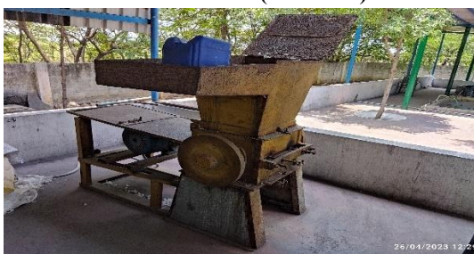
Shredder for shredding Plastic Waste at Athivaram village
