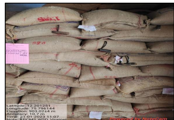
Extensive use of manual hooks on the gunnies lead to spillage of grains - APCMS Virajpet, Kodagu
