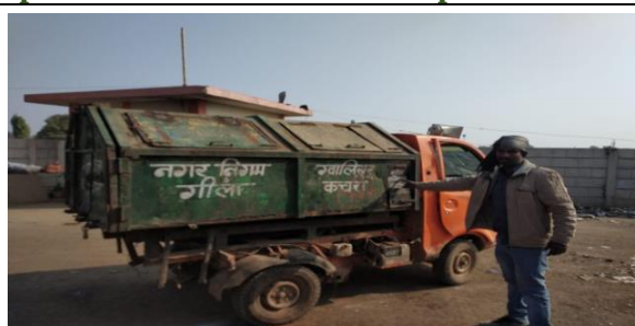
Image 2.21: Collection vehicle without separate boxes for special wastes ULB, Gwalior
