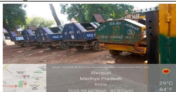
Image 2.20: Vehicles without separate boxes for collecting domestic hazardous waste in ULB, Shivpuri
