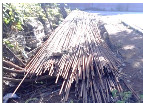
20 mm TMT steel bars (Thoubal Project)
