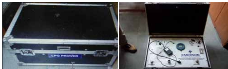
Photograph 4: CNG/LPG dispensers verification kits
