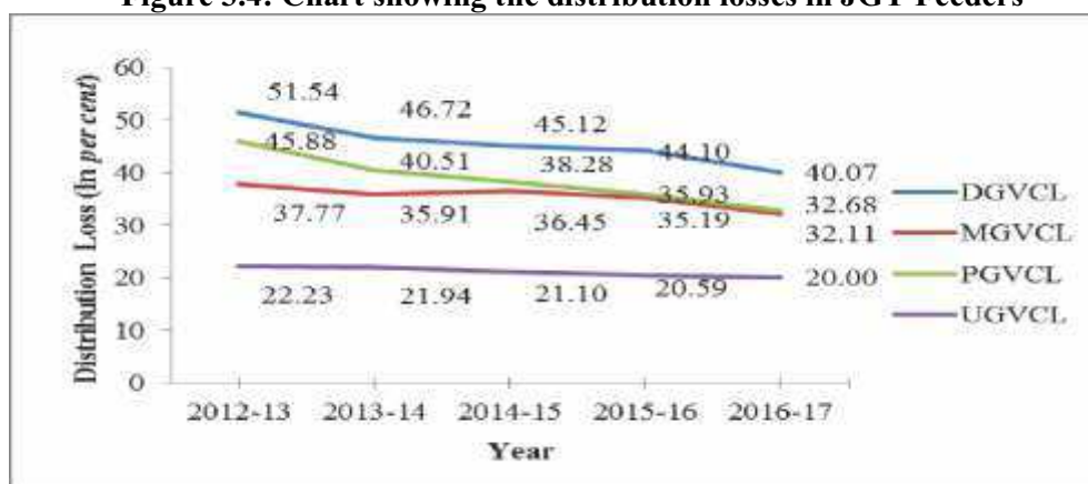
Figure 3.4: Chart showing the distribution losses in JGY Feeders
