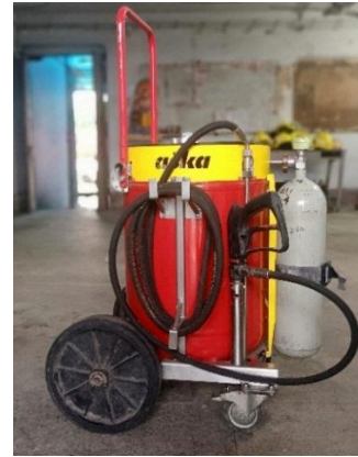
Pic 3.5: Trolley mounted Foam Drum
