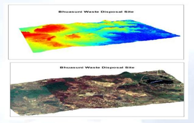
Image 2&3: Digital Elevation Model of the Bhusani Waste Disposal Site (2) and Satellite imagery superimposed for the site (3) [Height exaggerated for better visual representation]
