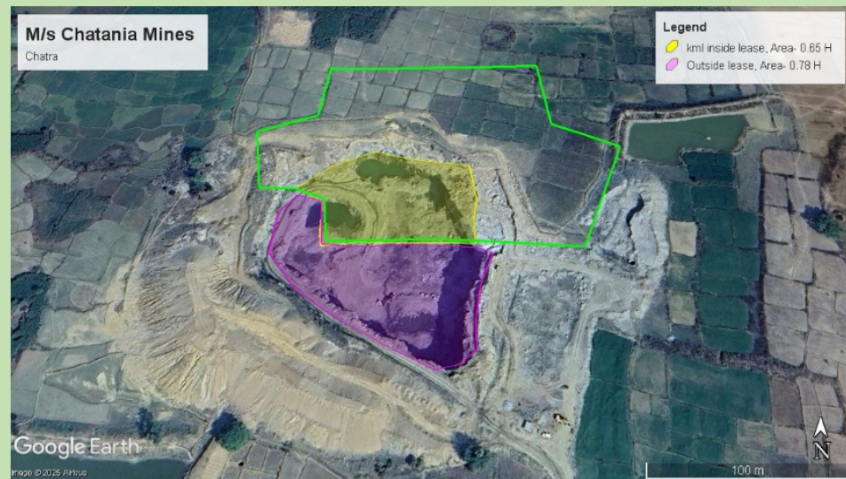
Picture-4.21: Google Image (17 February 2022) showing lease area (kml area 2.83 Ha.) outlined in green, excavated area inside lease area shaded in Yellow (0.65 Ha.) and outside lease area in purple colour (0.78 Ha.), Depth measured in JPV (23 May 2023): (39.90 meter against permissible depth of 20 meter)
