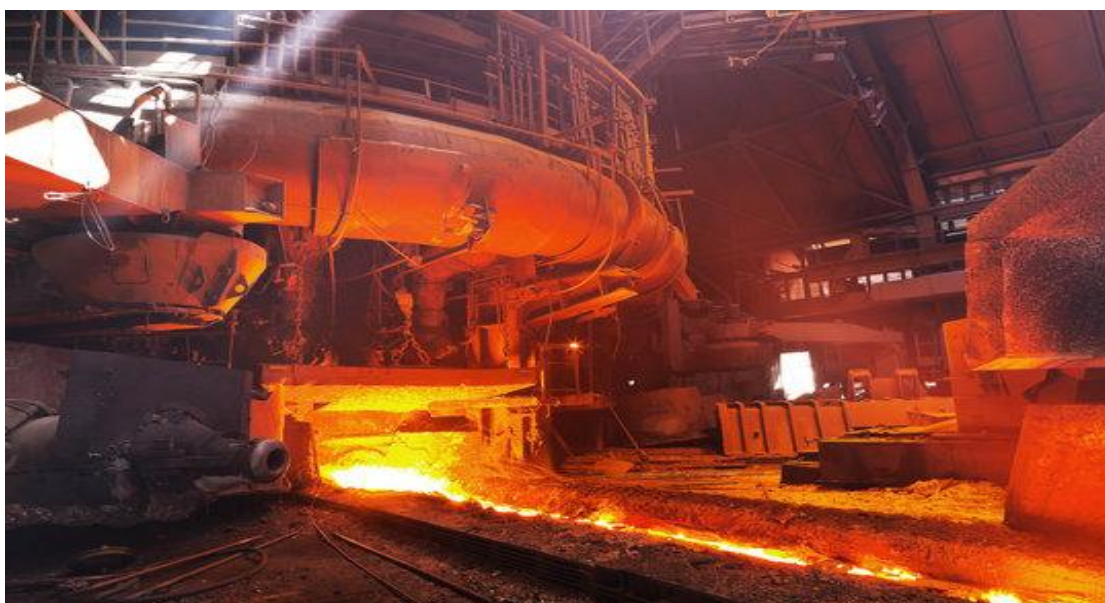
Figure 6: Hot metal flowing through main trough from BF#8 of Bhilai Steel Plant
