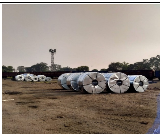
Figure 6.12: Cold Rolled Coils lay in open area at Durgapur Stockyard
