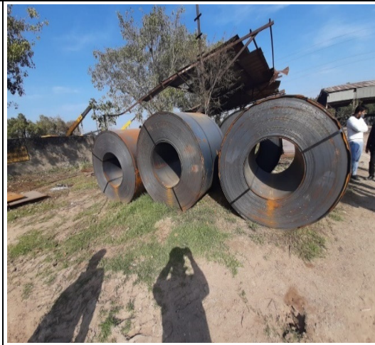
Figure 6.6: Material without dunnage at Chandigarh
