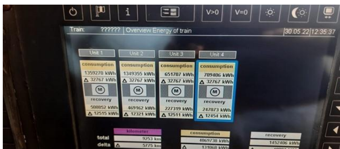
Image 2: EMU metering panel showing energy consumed and regenerated
