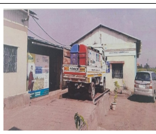
Photograph No. 4: Weighbridge at the entry point of dumping ground in Malkapur MC (February 2021)
