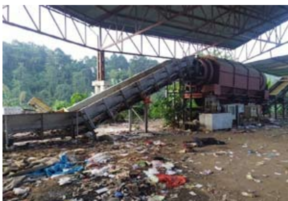
Exhibit 6.7: Compost Plant Machineries with vegetation coming up at Nongpoh
