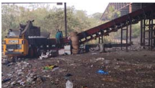
Exhibit 6.15: Mixed waste put into first input section of the compost plant
