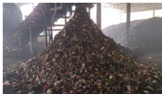
Exhibit 6.16: Output from the first section not properly segregated
