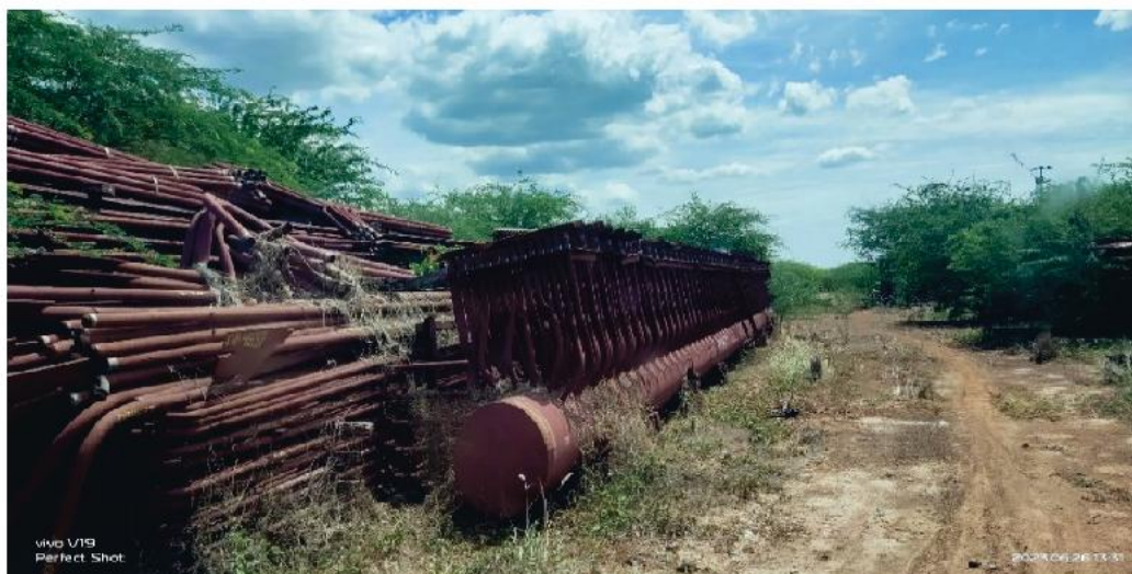
Picture 1: Cooling water pipelines kept in open, surrounded by bushes.
