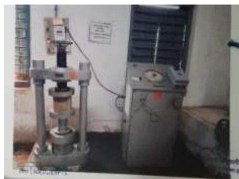
2. Compressive strength Testing machine Dated: 04.10.2021(Janjgir lab)
