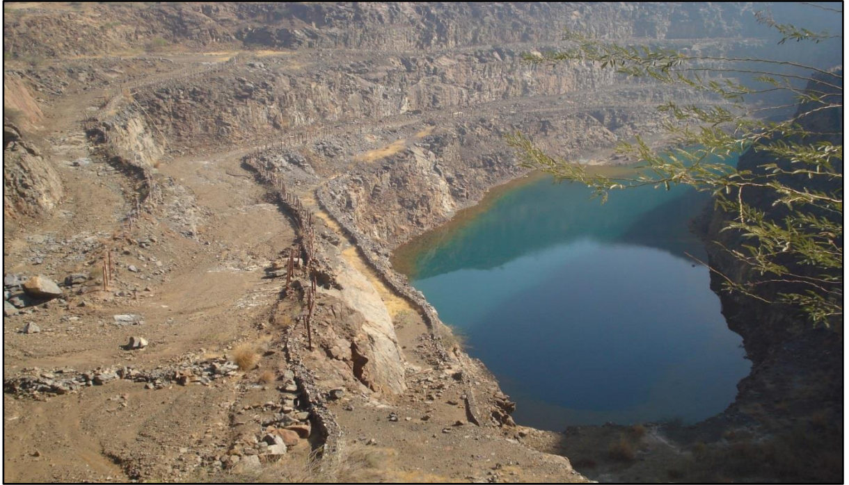
Figure 3.2: Benches of Chandmari open cast mines
