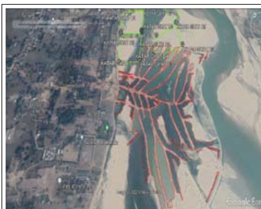
Figure 85: Plotted mined area in red boundary in Katar sand ghat extraction measured in January 2019.
