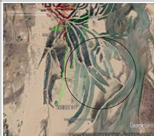
Figure 61: Outside extraction shown in May 2019 at Darihat 3 sand ghat.
