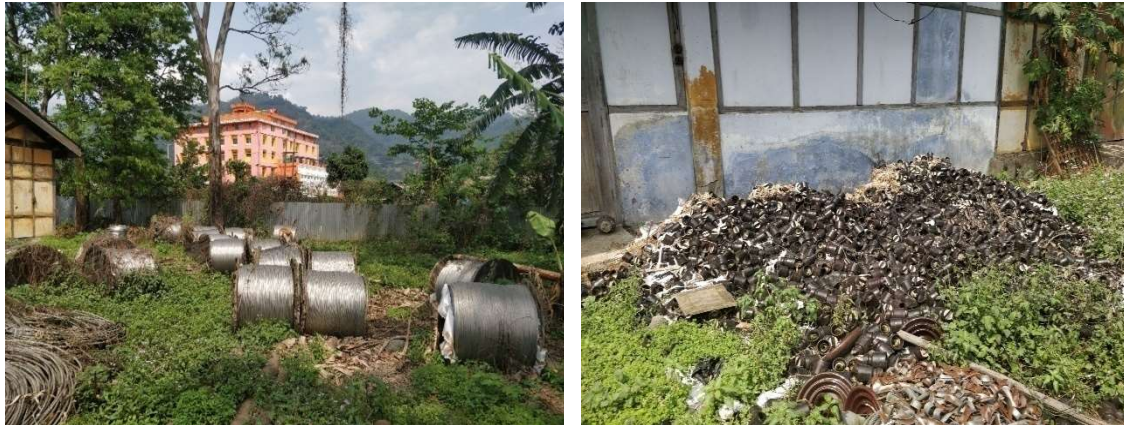
ACSR Conductor (Squirrel) and LT Pin Insulators lying unutilized at Roing Divisional Store
