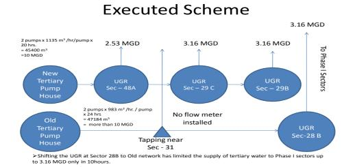
Audit is of the view that shifting of UGR at Sec 28B from new distribution network to old distribution network, changed the thrust of the whole project:
