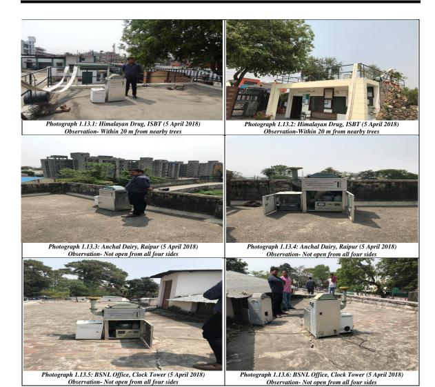
Installation of the air monitoring instruments in contravention to the prescribed norms has the risk of generating inaccurate and non-representative result.
