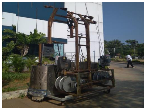
Exhibit 3.7: Carriage of Facade Access System
