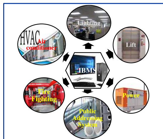
Exhibit 3.6: Illustrative diagram of IBMS
