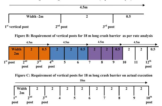
Figure A: Length of 4.5 m crash barrier (as per rate analysis)
