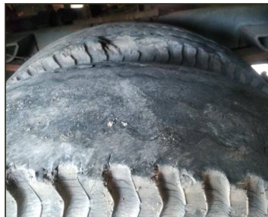
Picture 4 : Poor tyre condition, Bahour fire engine
