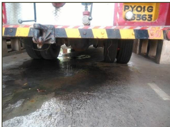
Picture 3 : Intense water leakage, Karaikal fire engine
