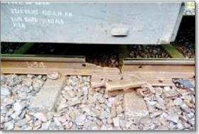
Figure 4: Rail fracture
