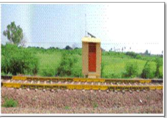
Figure 6: Wheel Impact Load Detector
