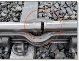
Figure 5: Weld failure
