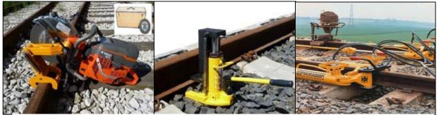
Figure 8: Abrasive Rail cutter
