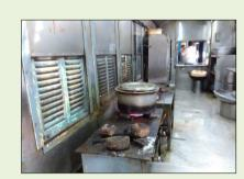
Fig. 1: Use of open flame gas burner in Train No. 12955 Mumbai Central - Jaipur Superfast Express (07.10.2016)
