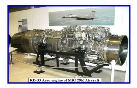
Audit observed (December 2014) that as of September 2014, a total of 65 engines (42 with 21 aircraft and 23 spare) had been accepted. However, since induction in February 2010, 40 engines (representing 62 per cent of 65 engines) had been withdrawn from service/rejected due to design related defects/deficiencies. The issue had serious flight safety implications, since in-flight engine defects had led to ten cases of single engine landings.
