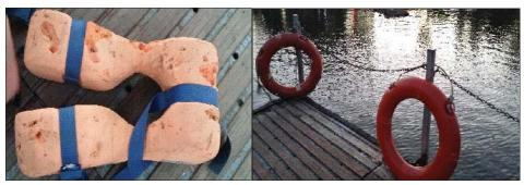
(Photos of Torn life jacket and safety ring tied with wooden platform at Saputara lake)
