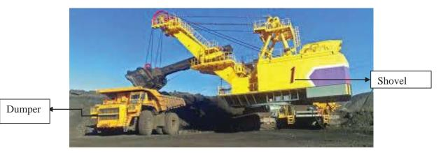
The Company had carried out (January 2011) a cost benefit analysis in cases where the depth of quarry was more than 100 metres or lead distance four KM or more. A combination of five cubic metre (CUM) Shovel with a 60 Tonne (T) dumper was found to be more economical (by  $\gtrless$  6.68 per bcm) than the combination of three cum Shovel with 35 T dumper.
