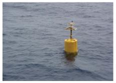
Spar type low cost buoy
