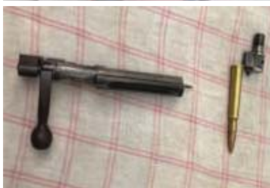
Glimpse of a defective pin and ejector
