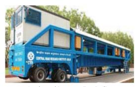
Accelerated Pavement Test Facility
