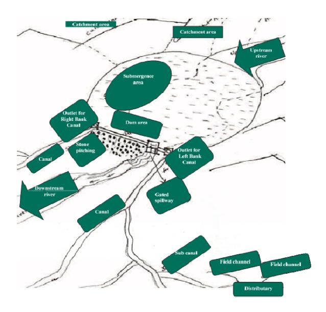
**Dam**: A dam is a wall of solid material built across a river to block the flow of the river. The continuous flow of water from the river upstream of the dam accumulates in the reservoir formed upstream of the dam. Depending on the purpose, water from a dam is released into canals for irrigation purpose or into pipelines to supply water to a city or to a hydro-electric power station to generate electricity. Excess water in the storage reservoir is released through
