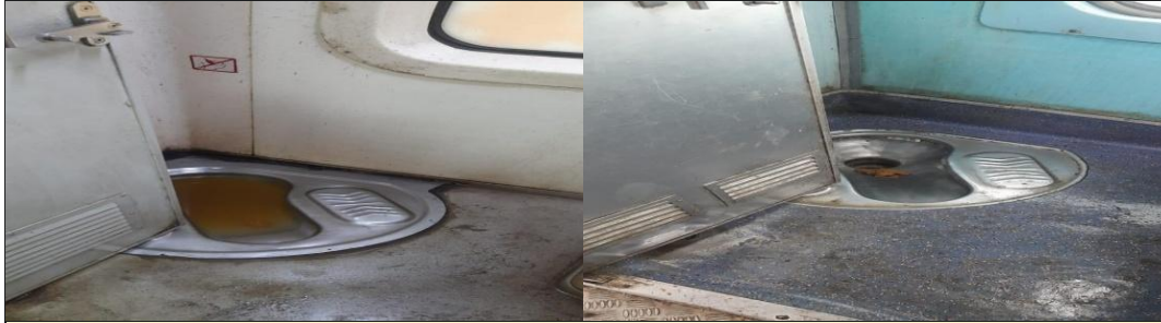
Choked toilets of sleeper coaches of train 19019 at CTS Ratlam of WR
