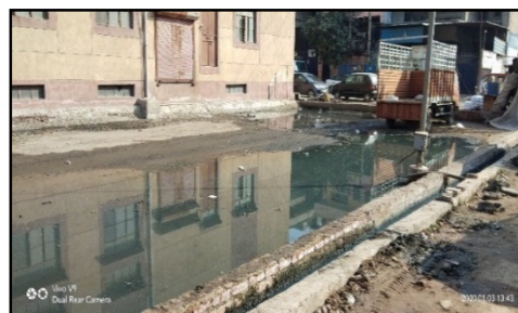
Photographs 4 and 5: Choked drains and overflowing drains in Narela IA, as observed during joint physical verification in January 2020
